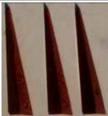
Pyrometric cones (for measuring the temperature in the kiln)
